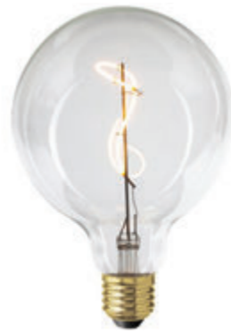
DL120 E27 4W 130 lm 2200K energy class A+ vetro chiaro clear glass dimmerabile dimmmabile h 145mm Ø 125mm
